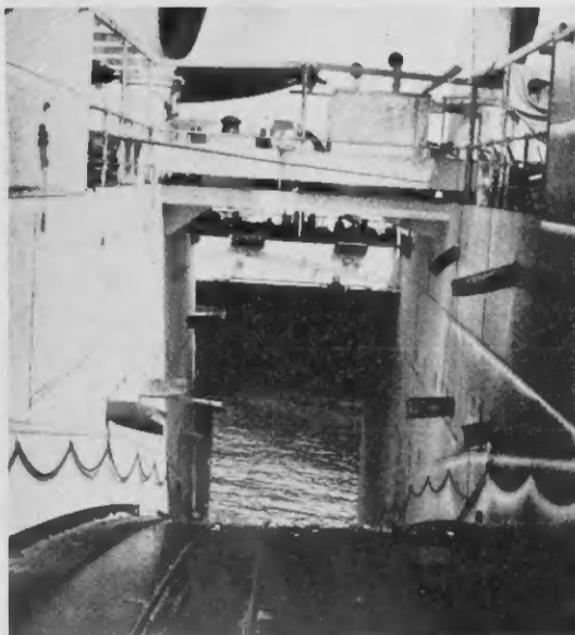
THE WHALE is hauled out of the sea through a large opening in the factory's stern, left. A veteran shows a neophyte how to fit a killer bomb on a harpoon shaft. The bomb contains 150 grams of powder.
